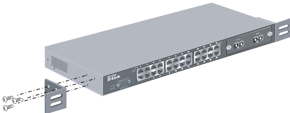
Figure 2-5. Attach mounting brackets
